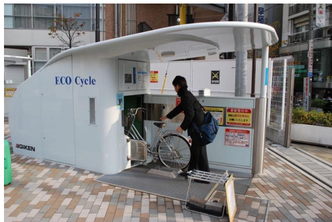
Figure 28: Entrance to automated underground bicycle parking (Asano, 2017)
