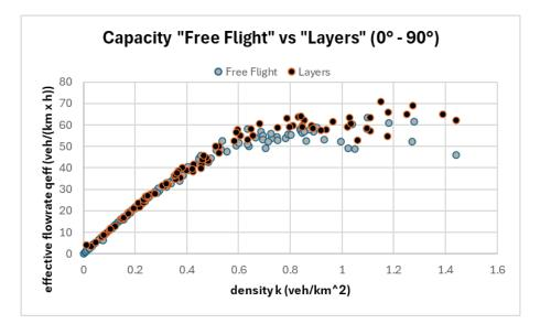
**Connection between road network and air network capacity:** Road networks and air networks behave similarly, as can be implied by the resemblance of their fundamental diagrams (diagram of autobahn observations on the left). The capacity increases until the point of critical density. If the critical density is surpassed, capacity starts to decline. Calculations of the optimal speed (slope of the green line) for the critical density imply that aircraft move faster than cars at that density.
