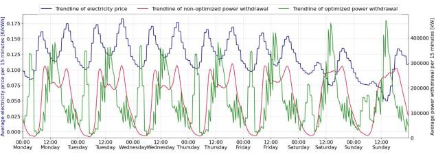
optimization approach is based on shifting power withdrawal to time periods of minimal electricity prices within the vehicle's connection time. This is visualized by the diagram above, where the blue line represents the electricity price, the red line the non-optimized power withdrawal, and the green line the optimized power withdrawal over the average week of the study period.
